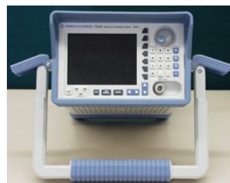
2. Slide the handle lengthwise while twisting it radially in steps of about 12°.
