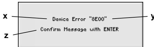
The error number allows the service shop to determine the type of error. In the event of a system message, please write down the error number and proceed according to the following steps.
