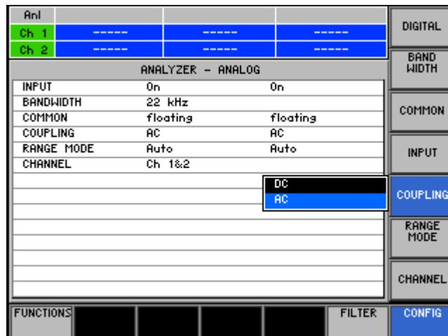
4. Select a signal coupling with **rotary knob** [11].
